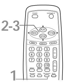
**Press REW/**◄ or **F.FWD**/►. The TV/VCR will rewind or fast forward the tape by the specified amount of time. The time counts down on the screen as the search progresses. When 0:00 is reached, the tape will play automatically.
